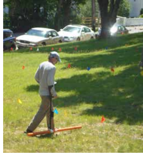
Figure 15. Survey in process: left) GPR surveying with the Mala X3 equipped with a 500 MHz antenna; right) FDEM surveying with the CMD Mini-Explorer.
