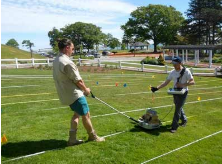
Figure 15. Survey in process: left) GPR surveying with the Mala X3 equipped with a 500 MHz antenna; right) FDEM surveying with the CMD Mini-Explorer.
